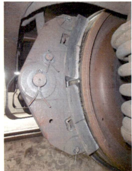
Melted brake block
