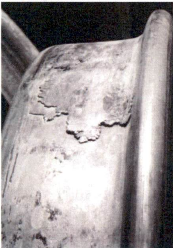
Metal build up on the tread
