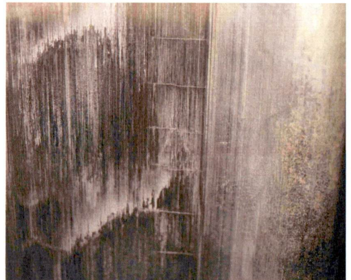
Example for single cracks on the wheel tread by visual inspection
