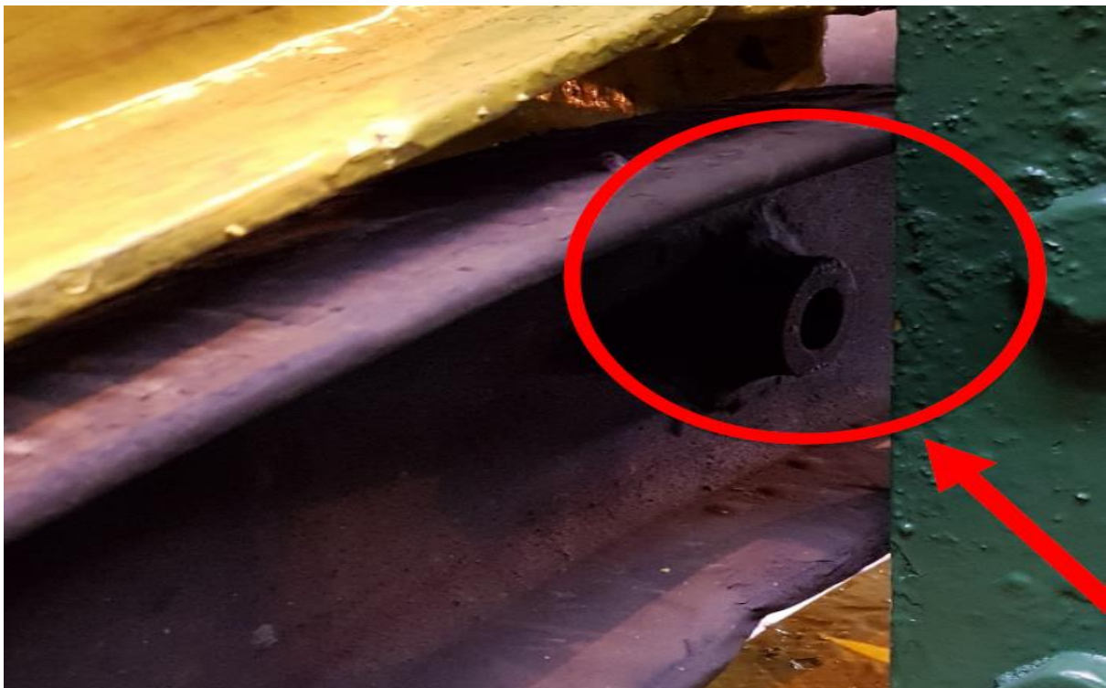
Picture 4. A characteristic point of bogie frame of ARAD Romania production – centering sleeve located on the frame end.
