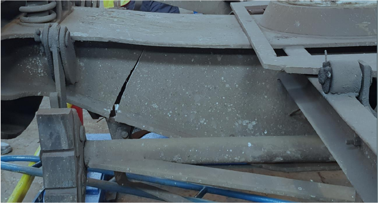
Picture 1. View of the crack at the lower belt of bogie's torsion beam.
