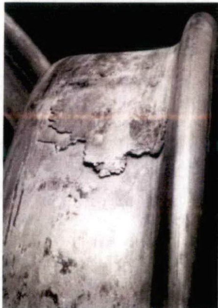
Metal build up on the tread
