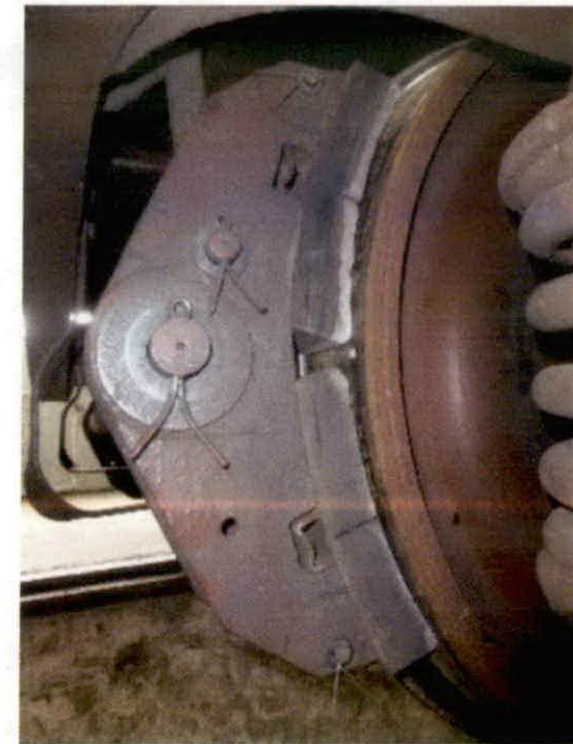
Melted brake block
