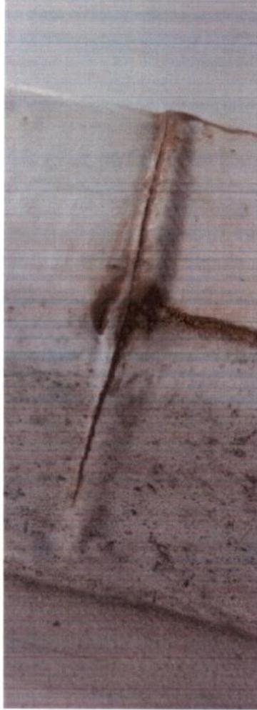
Attachement with e-mail dated 16th March 2018 concerning cracks in the stiffeners ring of type Z23A tank wagons series Zacns, capacity 87m3 ans Z24A, tank wagons series Zacns of 97 m3
