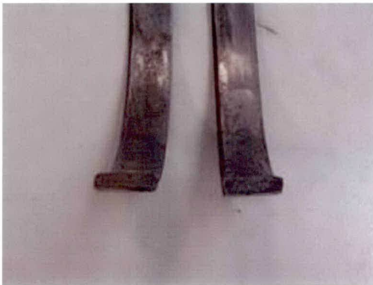
Wear of the locking ring around the load bearing corners
