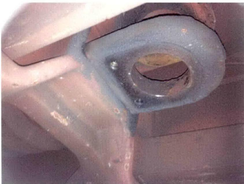
The hook pin failed and the washerplates was not bend properly.
