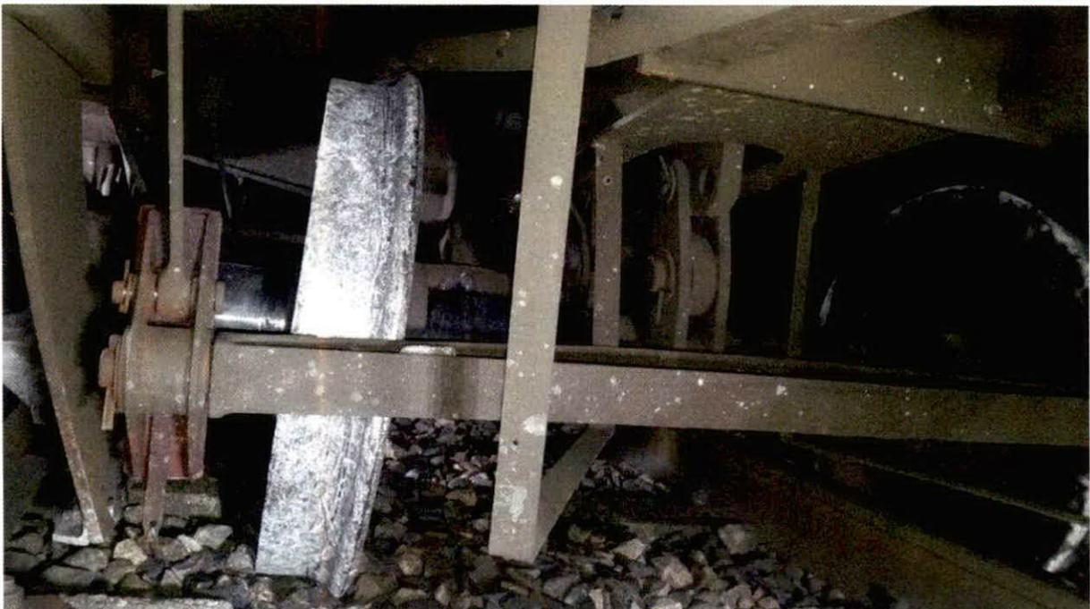
The wheel plate broke radially from the wheel tread to the centre of the wheel:
