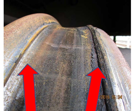
Extraordinary wheel tread deformation on the outer side of the tread and near the flange
