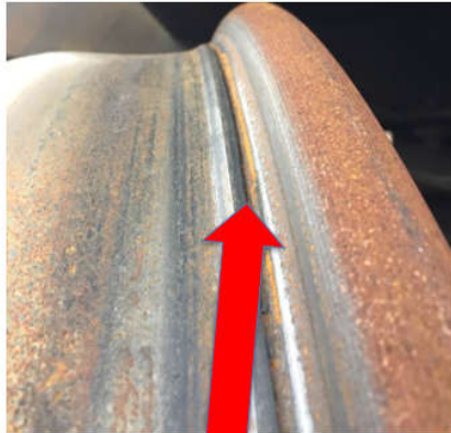
Extraordinary wheel tread deformation near the flange
